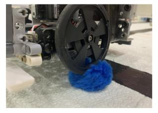
The presence of obstacles on the game table poses a further threat to the robots. Most of the time, a properly installed bumper can push away dangers in the robot's way, but sometimes, deformable objects, such as pom balls, can be squashed and slide under the bumper. The wheel would slip if a pom goes beneath it, and this causes the robot to deviate off course. Interference from the opposing team can also similarly affect the robot's movement.
